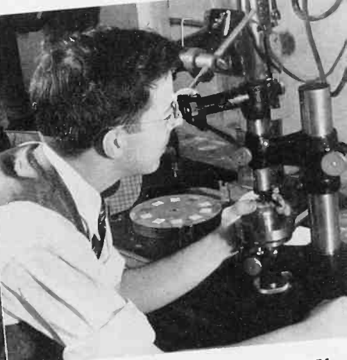
GROOMED for same frequency, groups of plates are lapped together. Required flatness and thickness are attained to an accuracy of 20 millionths of an inch.
