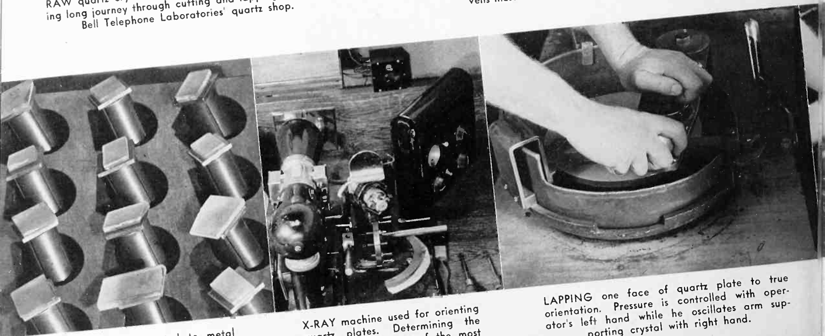
ROUGH blanks cemented to metal holder await their turn to be oriented under x-ray machine. This is one of many axes test crystals must undergo.
