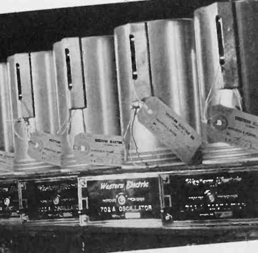
LINE-UP —702A oscillators awaiting 7A quartz plates which will control frequencies of various broadcasting stations.
