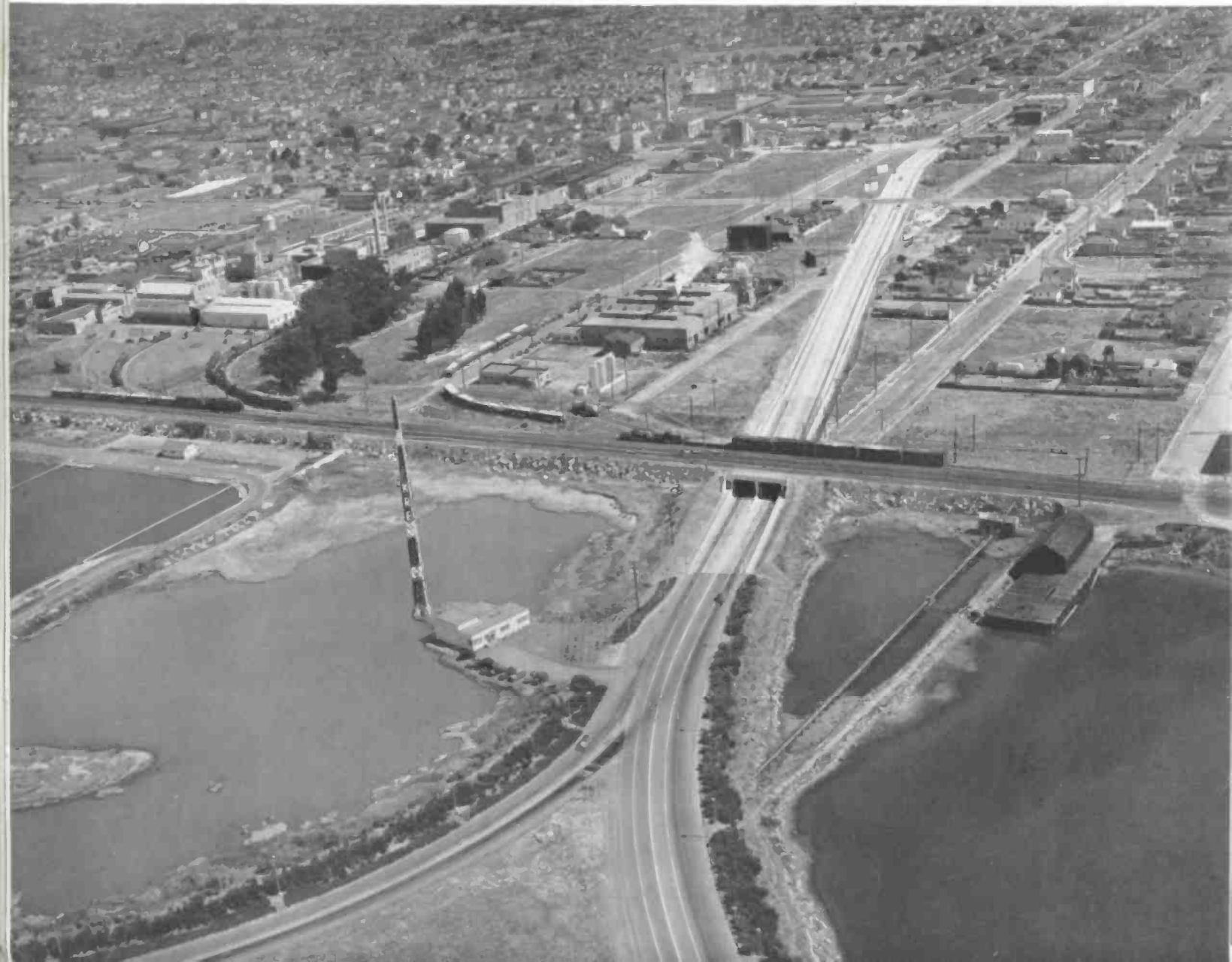
Aerial view of 250 watt AM Station KRE, Berkeley, California, with combined transmitter-studio building, shows a site with many advantages. Transmitter is on edge of community, with easy access by main highway. Sheltered body of water provides excellent grounding conditions.
