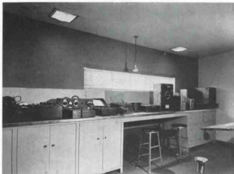
Workshop at WTOP has ample bench space with covered storage below the bench. Note natural and artificial lighting over working area.
