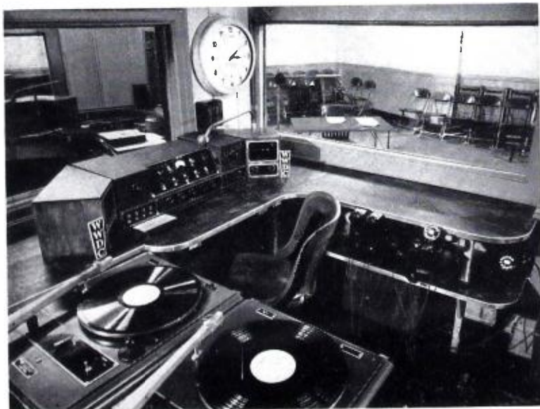
Control room at WWDC and WWDC-FM has view of two main studios. Transcription equipment in foreground is within easy reach of operator.
