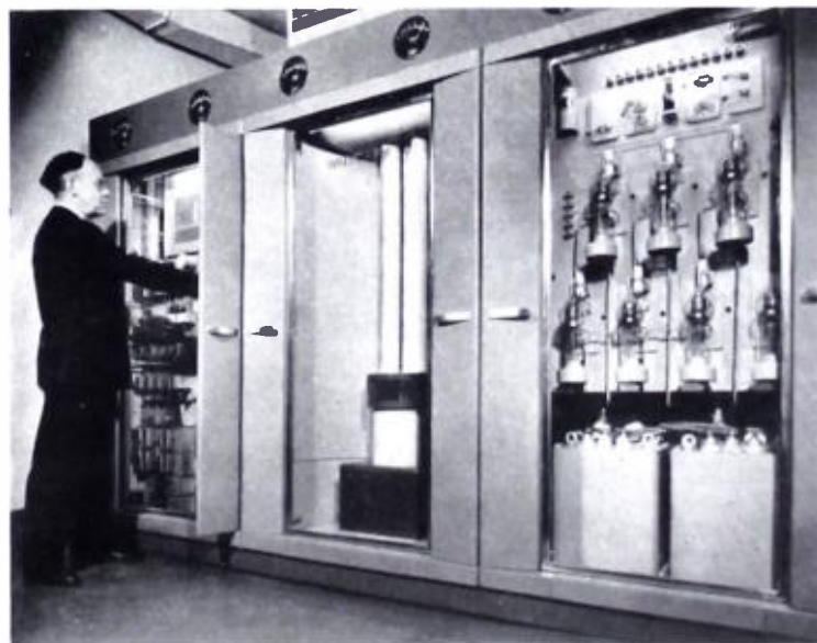
New 10 kw FM transmitter at WNYC-FM is adjusted by Chief Engineer W. H. Pitkin. Municipal station got full power on FM February 11, 1948.
