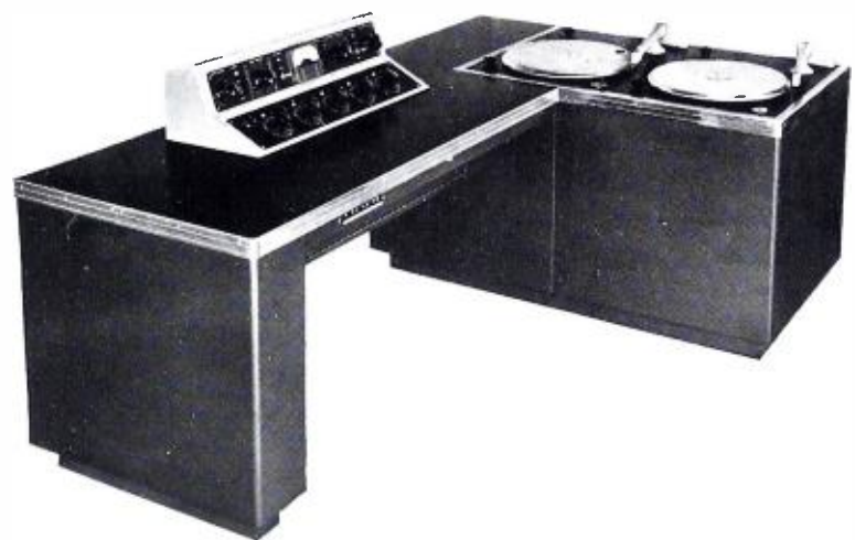
Above is the studio type transcription console, showing the convenient placement of the transcription tables at operator's right hand.
