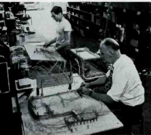
Operations for motion picture recording system are similar to those required in constructing audio facilities for broadcasting. Here is wiring form.
