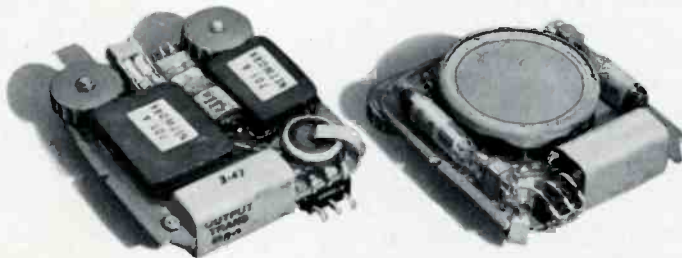
Figure 2 — Two views of amplifier chassis of Model 66 Hearing Aid. Left are moistureproof blocks containing interstage coupling networks, one tube, tone and volume controls; at the right are microphone, two tubes and transformer.
