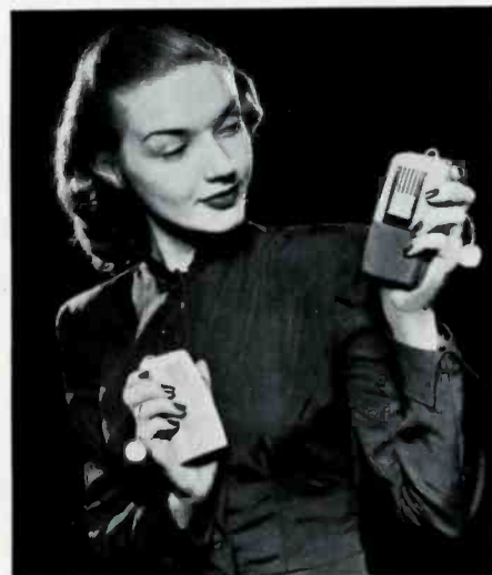
Held in the right hand is Hearing Aid Model 65, designed for persons with moderate hearing losses; in left hand is the Super 66 with a high power output for persons with severe hearing losses.
