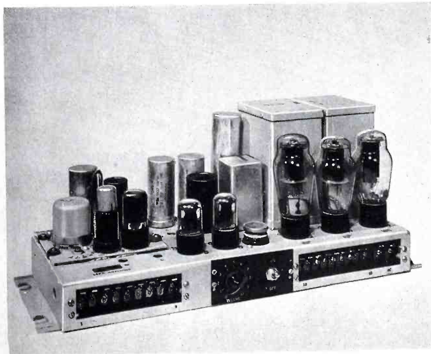
The 142B Amplifier has 25-watt power output, with dual line-level input, master gain control, and includes a 141A as a preamplifier or booster.
