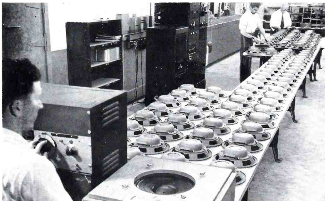
Loudspeakers lined up for the sweep-frequency noise and rattle test, carried out by the operator in left foreground. The automatic recorder for the final frequency response test is in the middle background.
