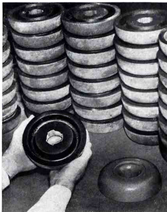
Unusually large magnet of Alnico is used in new 728B speakers to assure efficiency and quality.
