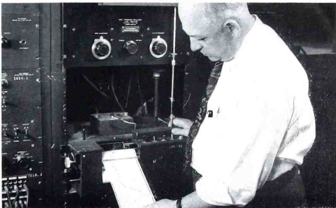
Automatically recorded graph showing frequency response of a completed loudspeaker comes off the machine specially designed by Western Electric to make this final quality test of the manufacturing process.
