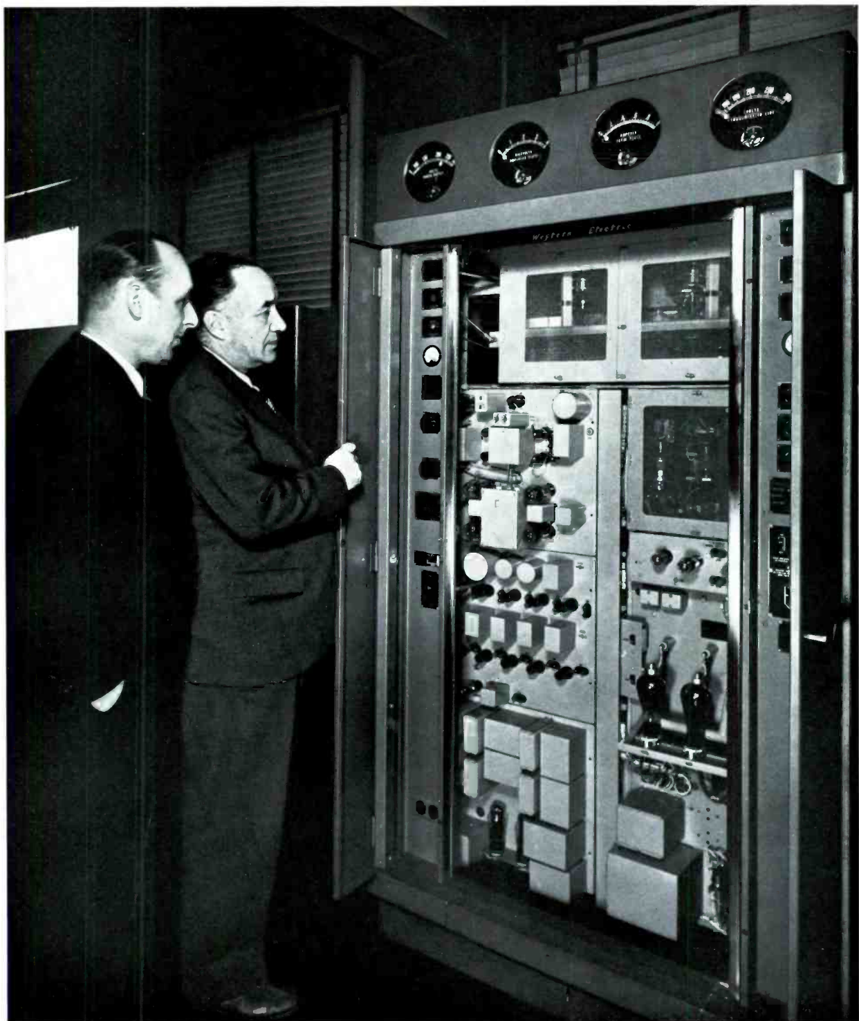
Station WELL-FM, Battle Creek, Michigan, is first to install Western Electric's new "Transview" FM Transmitter. Shipped direct from its preview at the NAB Con-
