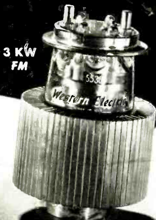
TYPE 5530 with terminal arrangement for grounded-grid application, as in Western Electric 3 kw FM transmitter.
