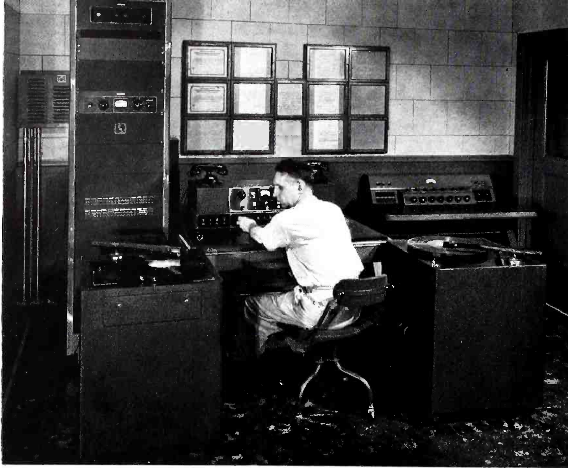
With one eye on the turntable, Grover Wizeman operates the 23C Speech Input Console at WMGM. The 25A Console in the right background will replace the 23C when the station's new 10 kw transmitter is installed.
