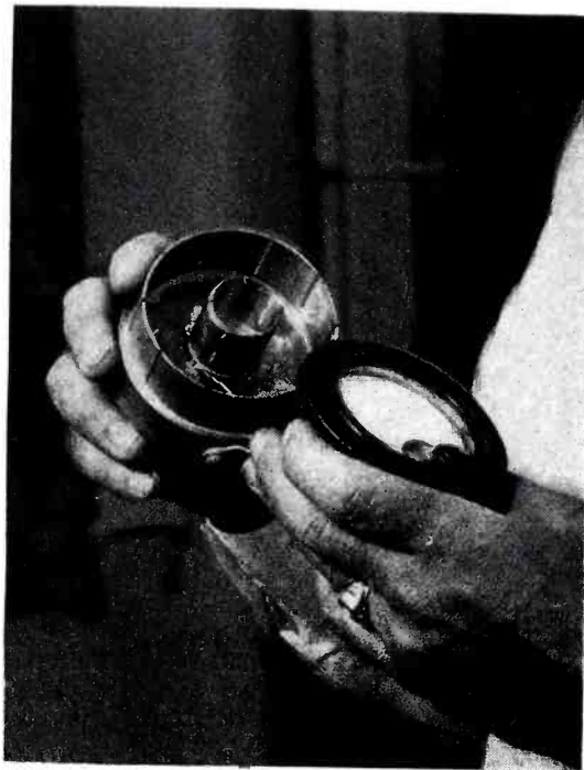
High frequency bridge for 3 1/8-inch coaxial line and its associated bridge detector current meter.
