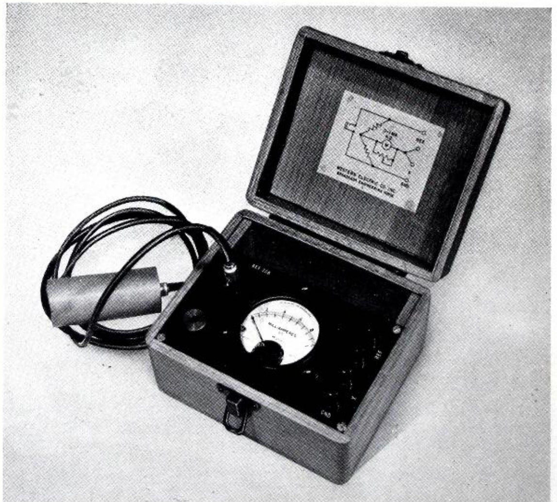
Reference type radio frequency bridge suitable for use on many of the tuned circuits found in radio transmitters of the modern types where a resistance requirement must be met. Bridge is simple and efficient.
