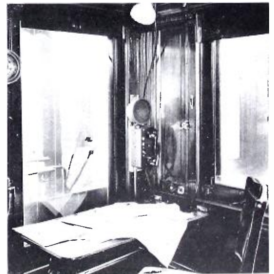
Radiotelephone handset and loudspeaker in business car, which was coupled to rear of 101-car freight and used in end-to-end test during an actual run.
