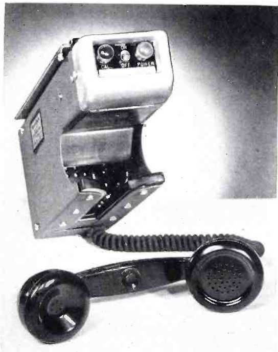
The 41A Control Unit is mounted under the instrument panel of the radiotelephone equipped vehicle.
