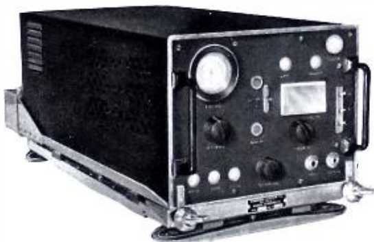
Naval aircraft radio, adapted from Western Electric commercial aviation radio telephone.
