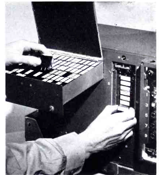
Figure 2. Crystal compartment and storage drawer for crystals not being used in transmitter.
