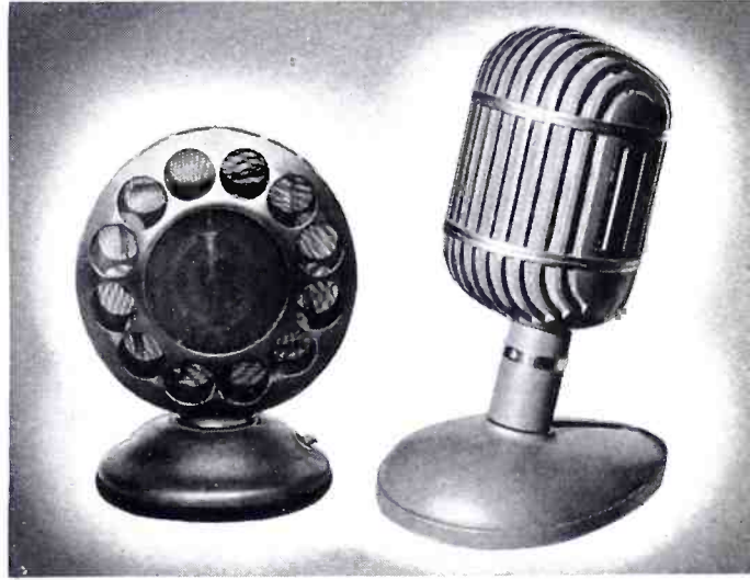
Western Electric "bird cage" carbon microphone made radio history, became symbol of broadcasting. The cardioid, developed just prior to war, is the company's latest and best. Many fine mikes came between the two.
