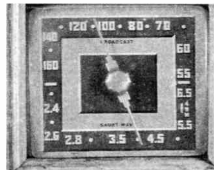
On this "split scale" dial, top of pointer indicates broadcast; bottom, short wave.
