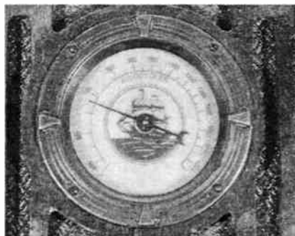
"Airline" dials had fixed scale, movable pointer, showed entire tuning range.
