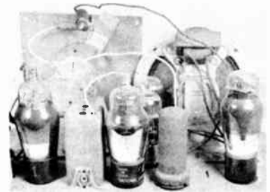
Tube heaters of a.c.-d.c. sets are in series. Ballast resistor, if present, looks like a metal tube (see text).
