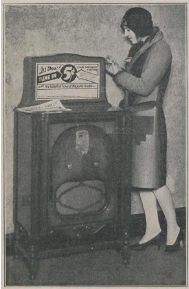
Figure 1: Set-top coin-operated radio timer
