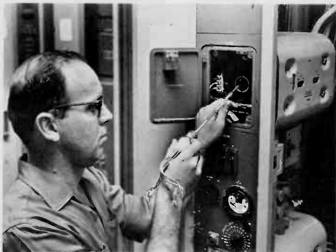
TRAVELING-WAVE TUBE, shown here in the hands of a telephone technician, is the amplifying device planned for use aboard Bell System's proposed satellite relay station next year. The high-frequency micro-wave tube can amplify radio signals as much as 10,000 times.
