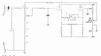
FIG. 9. The ac voltage measuring circuit. The condenser and resistor connected to the control grid of VT 1 in the diagrams are used to keep ac voltages from the grid.
