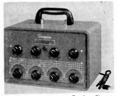
Courtesy Simpson Fig. 9. The Simpson Model 434 white-dot generator.
