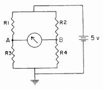
FIG. 2. A balanced bridge circuit.
