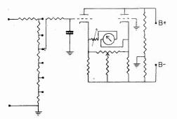
FIG. 7. The circuit change for measuring negative dc voltages.
