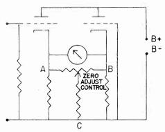
FIG. 4. The zero adjustment circuit.
