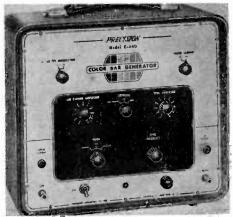
Courtesy Precision Fig. 8. The Precision Model E-440 color-bar generator.
