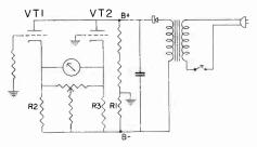
FIG. 5. The power supply circuit in the Model W VTVM.
