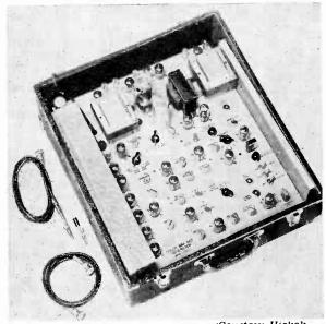
Courtesy Hickok Fig. 7. The Hickok Model 656XC color-bar generator.
