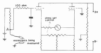
FIG. 8. The resistance measuring system.
