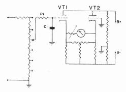
FIG. 6. The voltage divider. This permits measurements on various voltage ranges.
