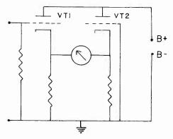
FIG. 3. The basic circuit of the VTVM. The ground connection in this and other diagrams is not a ground to chassis. It is a floating ground.
