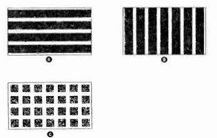
Fig. 4. Most white-dot generators will also produce the bar and crosshatch patterns shown here.
