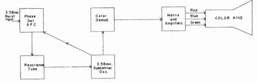
Fig. 5. Circuits that can be adjusted and serviced with a color-bar generator.
