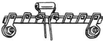
Fig. 2. The part leads may be wrapped around the lugs as many times as you wish. Most technicians use just enough of a wrap to mechanically support the part. Any excess lead length is clipped off after soldering.
