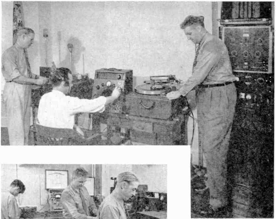
Above, Jay McCarthy, Wells and Jerry McCarthy show the set up they use in making a recording. When making "on the spot" recordings, this equipment is moved to the job. The microscope (partially visible behind Wells' head) is used to examine the cut on the recording.
