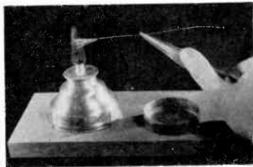
Fig. 3. If enamel covered wire is held just inside the tip of the inner cone of an alcohol burner flame, as illustrated here, the wire will become red hot and the enamel will burn off.
