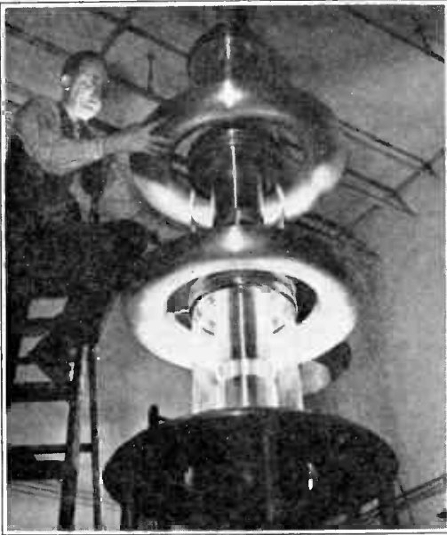
G-E X-Ray Tube, 1,400,000 volts, 10-section, 28.5 ft. Picture taken in G-E Research Laboratory at Schenectady, N. Y. Tube for National Bureau of Standards, Washington, D. C.
