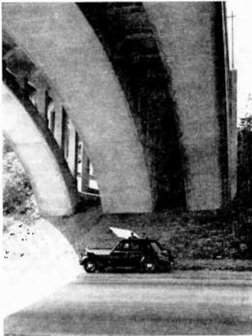
Under this bridge the AM signal from WOR took a nose dive, but W2XOR's FM signal came through loud and clear.
