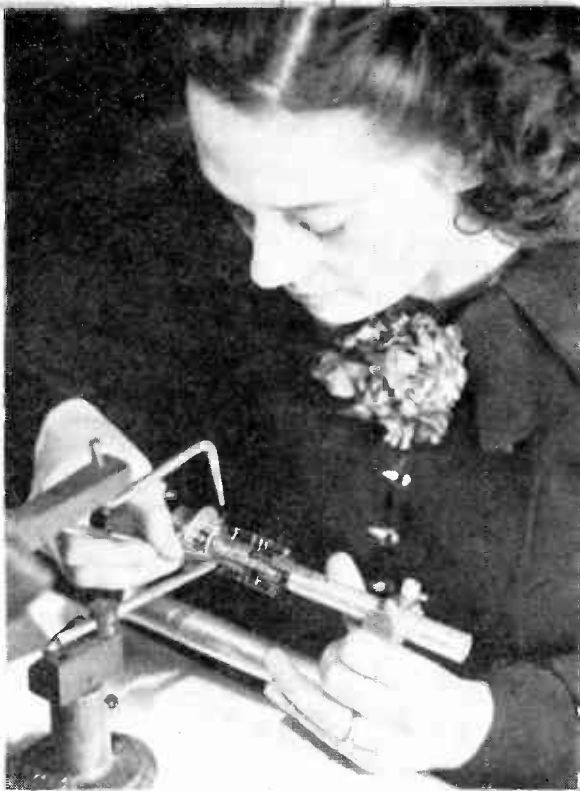
Fig. 6. Welding electrodes to base.
