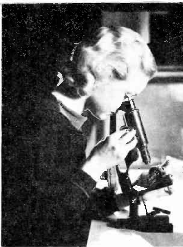
Fig. 5. Checking electrode alignment.
