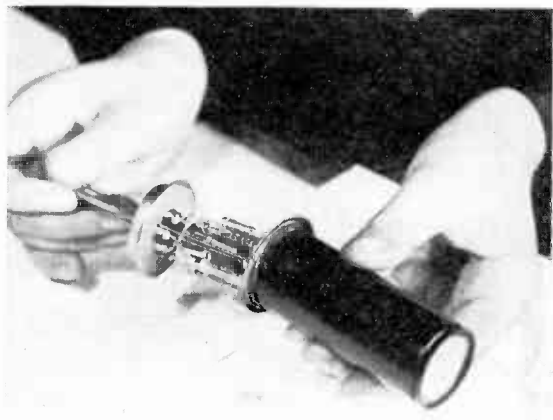
Fig. 3. (above) Assembling an electron gun. Fig. 4. (below) Assembling a type 913 tube.
