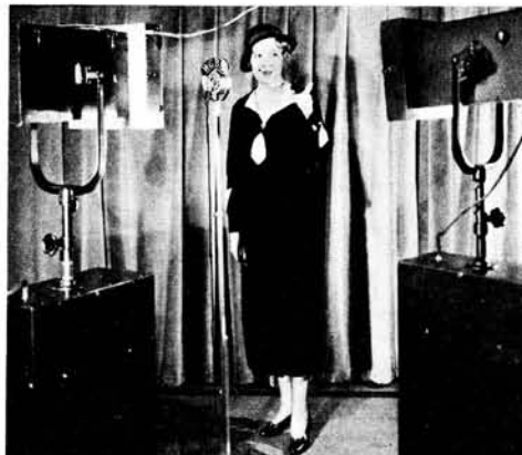
Using the flying spot direct pick-up at the Jenkins Television Station W2XCR. The boxes on each side of the object contain photoelectric cells and amplifiers.
