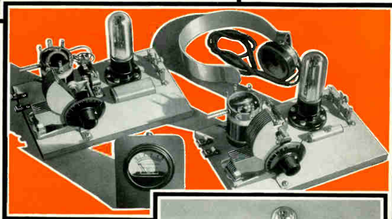
Tests conducted with modulated oscillator and detector.
