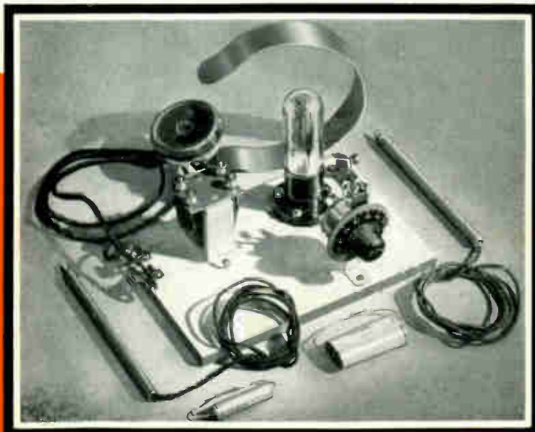
Practical testing equipment for measuring resistance, capacity and inductance with Wheatstone Bridge
