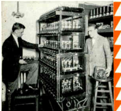
Over $60,000,000 worth of tubes were sold in 1931. This photograph shows two men testing tubes in a large manufacturing plant.
