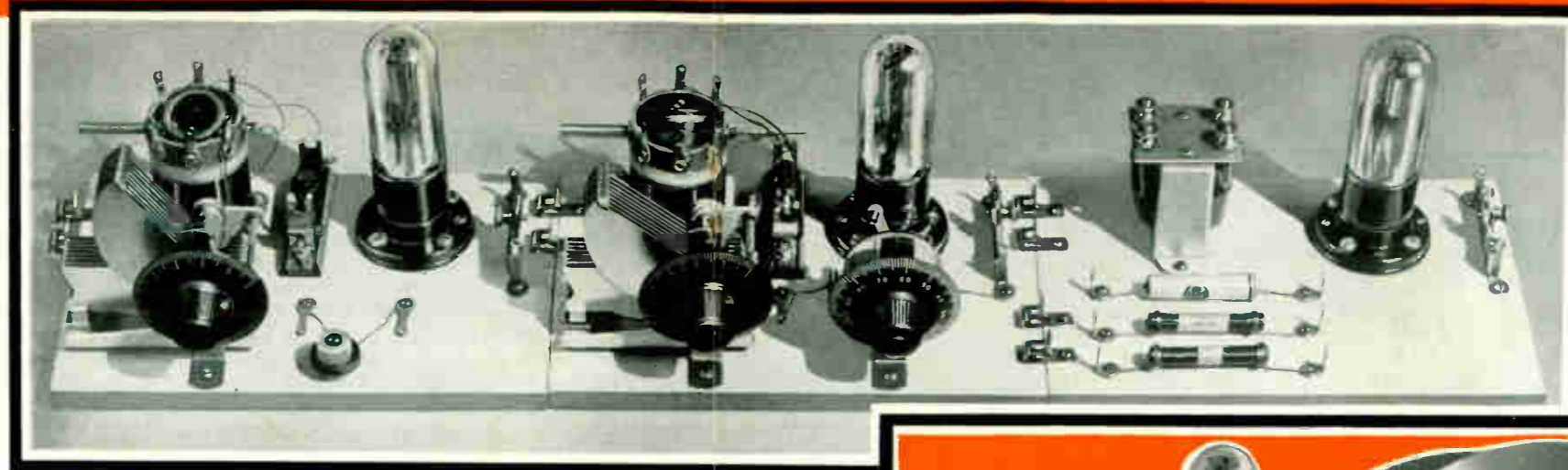
One stage of Radio frequency amplification, detector and one stage of audio frequency amplification for receiving signals.
