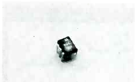
FIGURE 4. A TYPICAL OPTOCOUPLER.
