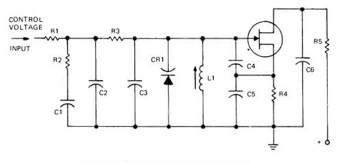
FIGURE 4. SCHEMATIC DIAGRAM OF THE VCO.
