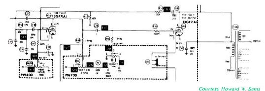
FIGURE 4. THE VERTICAL MULTIVIBRATOR AND OUTPUT CIRCUIT OF RCA CTC 51XAB/ CTC 52.
