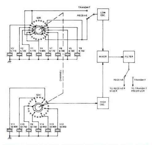
FIGURE 1. A MULTIPLE CRYSTAL FREQUENCY SYNTHESIZER USED IN THE JOHNSON MESSENGER 123A.
