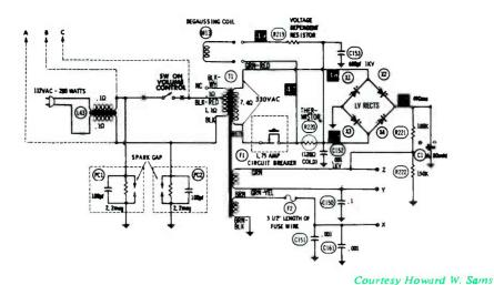
FIGURE 1. THE LOW VOLTAGE POWER SUPPLY AND DEGAUSSING CIRCUITRY OF RCA CTC 25.
