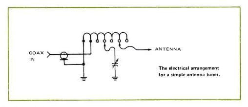
The tuner just described will handle only about 20 watts (the capacitor will arc), but you can use a transmitting type capacitor, a larger gauge wire in the coil, and then you can run much higher power. You must also have an SWR meter in the line from the tuner to the transmitter to make the thing work properly. This is an absolute must.
