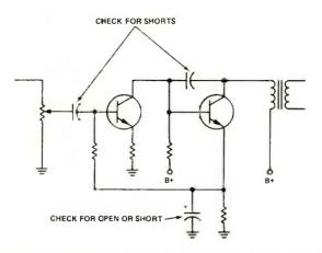
FIGURE & POINTS TO CHECK IN A TYPICAL AUDIO STAGE.
