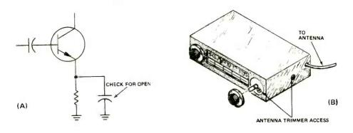
FIGURE 4. TESTING A WEAK RADIO.
