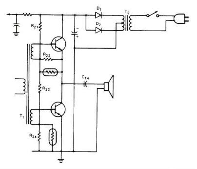
FIGURE 2. POWER SUPPLY AND OUTPUT OF TRUETONE GUITAR AMPLIFIER.
