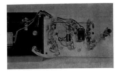
Fig. 3. Connections between top cover and box.
