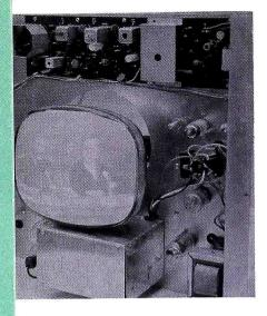
to test the permanence of your ections. When your work is done, k the high voltage in the customer's ne. This is the final step whenever you ice any color TV. Remember, imperly adjusted high voltage circuits luce not only poor pictures but also uble X-radiation.
