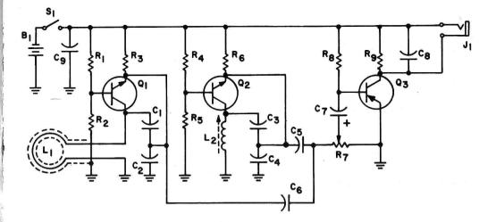
Fig. 1. Schematic of the metal detector.
