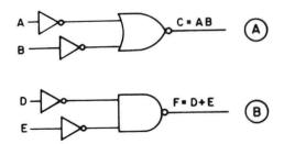
Fig. 6. Performing the AND operation with a NOR gate is shown at (A); performing the OR operation with a NAND gate is shown at (B).
