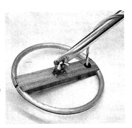
Fig. 5. The completed search coil attached to the exploring stem.
