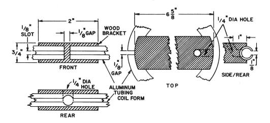
Fig. 4. Construction of search coil.
