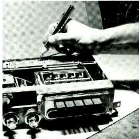
Fig. 3. A noise signal tracer is a quick way to locate a defective stage in the auto radio.
