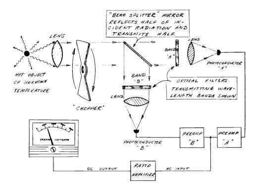
FIG. 9. Simplified color pyrometer.
