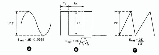
FIG. 3. Relationship between peak-to-peak and RMS for sine wave, A; rectangualr wave, B; sawtooth, C.
