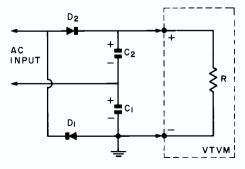
FIG. 6. Peak-to-peak probe for vtvm's.
