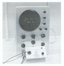
FIG. 10. Calibrator connected to produce 100V PP signal.
