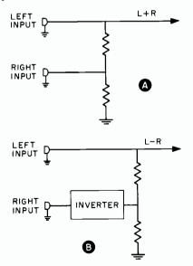
FIG. 2. Simplified matrix circuit.
