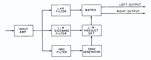
FIG. 7. Block diagram of FM multiplex adapter.
