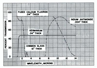
FIG. 6. Infrared transmission curves for various materials.
