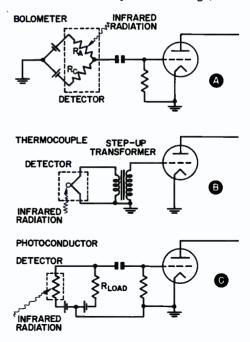
FIG. 4. Thermistor bolometer detector.
