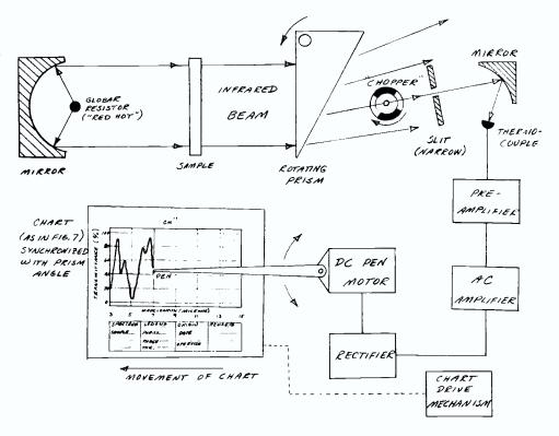
FIG. 8. Simplified infrared spectrophotometer.
