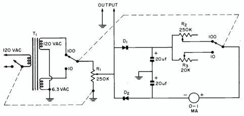
FIG. 8. Scope calibrator diagram.
