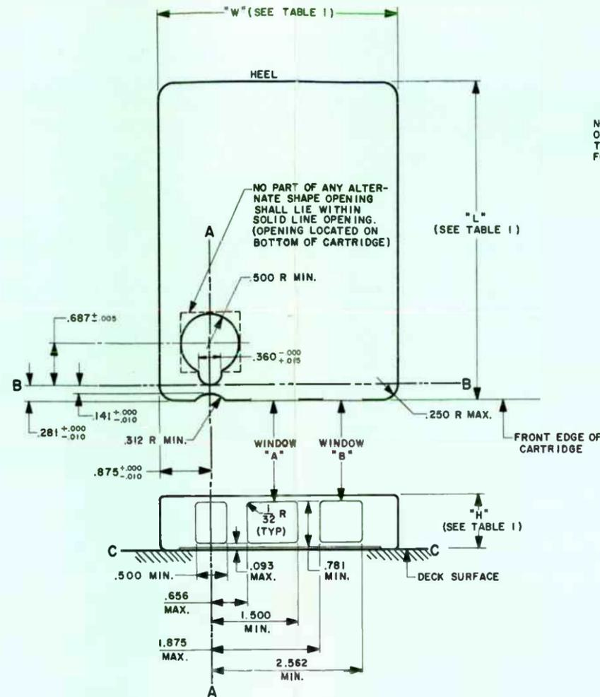
FIG. 3 CARTRIDGE DIMENSIONS
