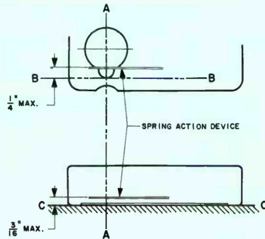
FIG. 1 REQUIRED SPRING ACTION DEVICE LIMITATIONS
