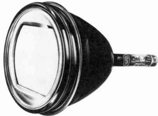
Fig. 2b: RCA 15GP22; first commercial shadow mask color CRT (1953)
