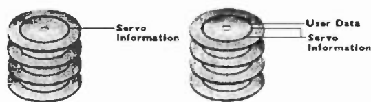
Figure 3 - Embedded versus dedicated servo
