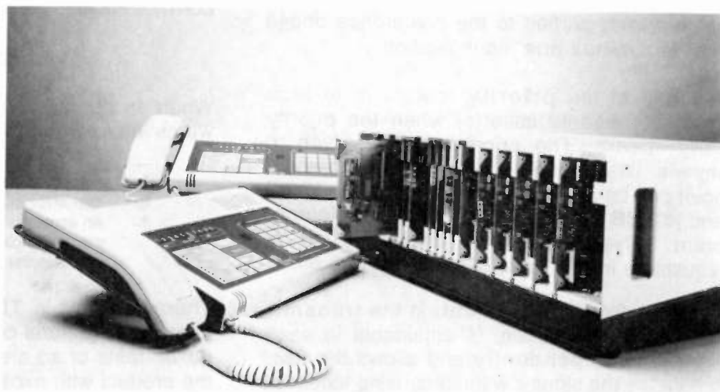
A system configuration of 2 control consoles and the CPU equipped with 5 double line cards in option (10 telephone lines)
