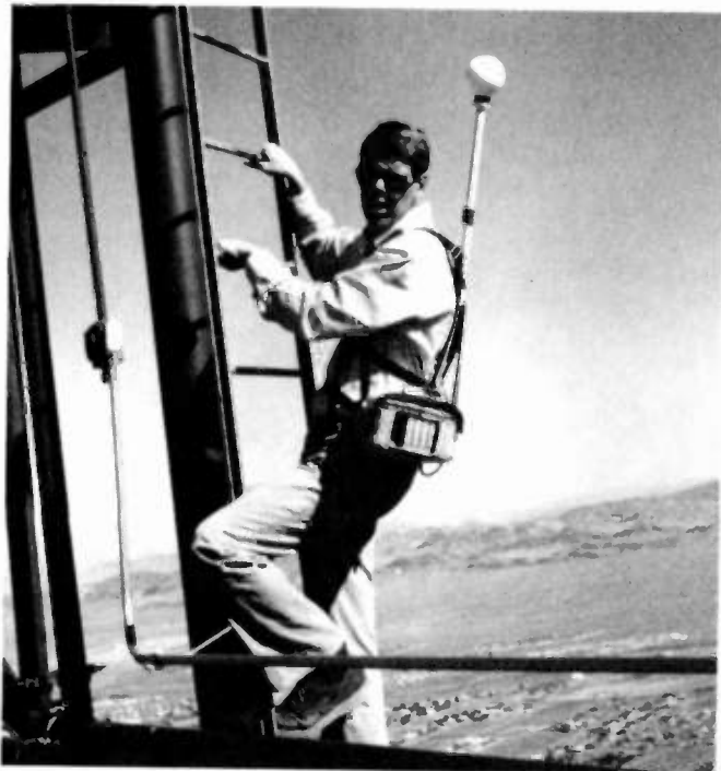
Figure 7. Using the portable measurement system for documenting time-averaged exposures during broadcast tower climbing. The system is being carried in a specially fabricated bag, similar to a camera bag, and the probe is supported above the climber's head by a harness assembly.
