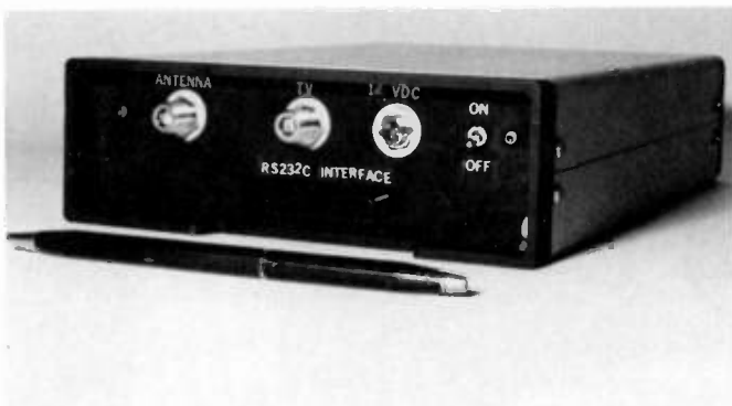
Radio Telecom Technology Inc. 2-way Radio Modem Prototype on TV Ch-6
