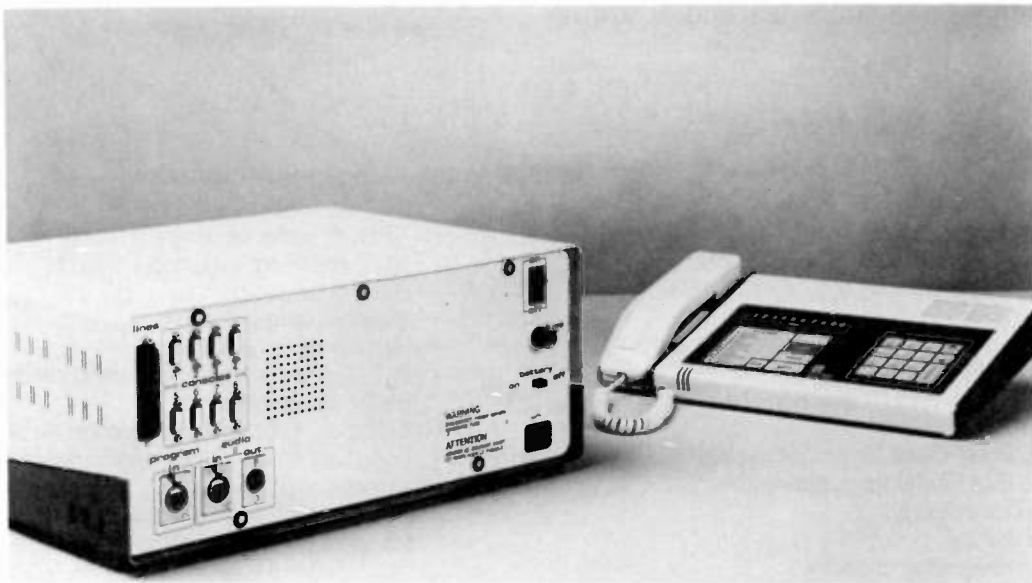
Rear view showing connectors (telephone lines, control consoles, audio)
