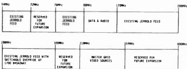
FIGURE 3. FREQUENCY ALLOCATION OF BI-DIRECTIONAL CABLE SYSTEM
