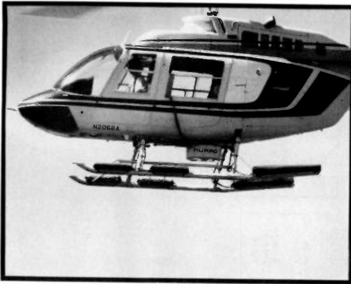
AIRBORNE VIEW OF SUPER POD INSTALLATION FIGURE 5
