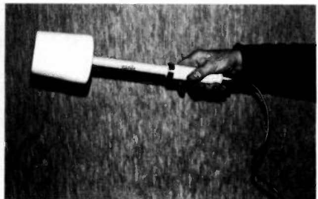
Figure 12. The same measurements with and without foil about the probe sensor is indicative of coupling into the potential field.
