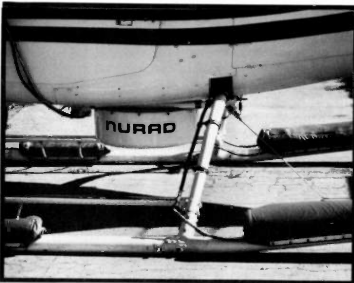
SUPER POD INSTALLATION SHOWING GROUND CLEARANCE FIGURE 6
