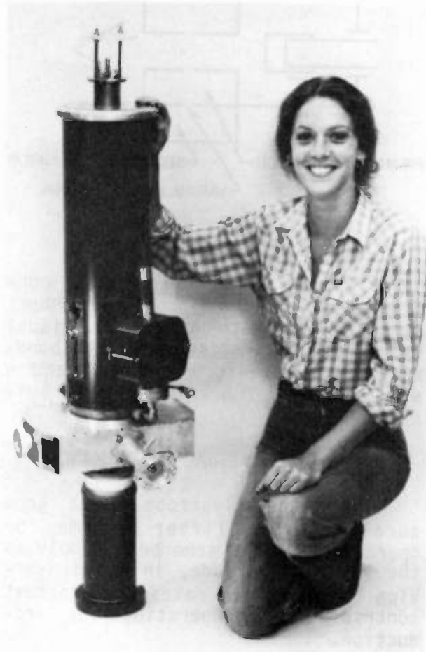
FIGURE 3 - KLYSTRODE WITH CIRCUITRY
