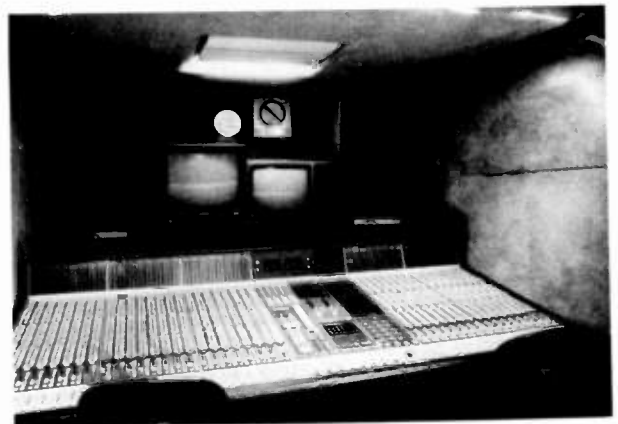
A Type A Vehicle - the 40 channel SSL Control Desk
