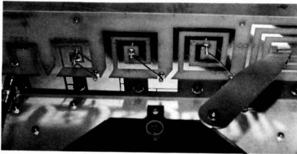
FIGURE 8. PHOTO OF INPUT MATCHING DEVICE. TUBE SOCKET GRID RING CONNECTION AT RIGHT OF CENTER, 50 OHM INPUT AT LEFT
