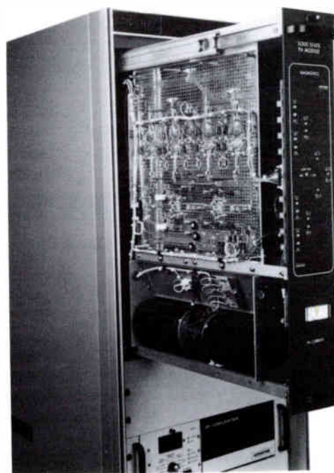
Figure 7. 250W Solid State Amplifier Module
