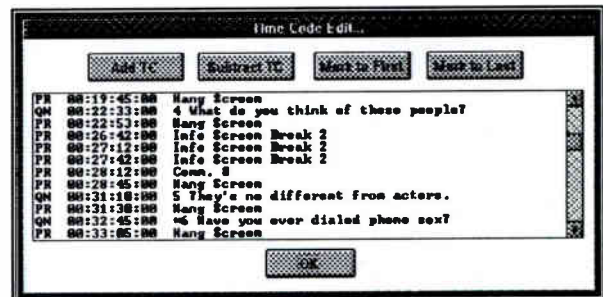
Time code can be modified to fit edit changes and then tested by playing back synchronous with video via a time code reader card.
