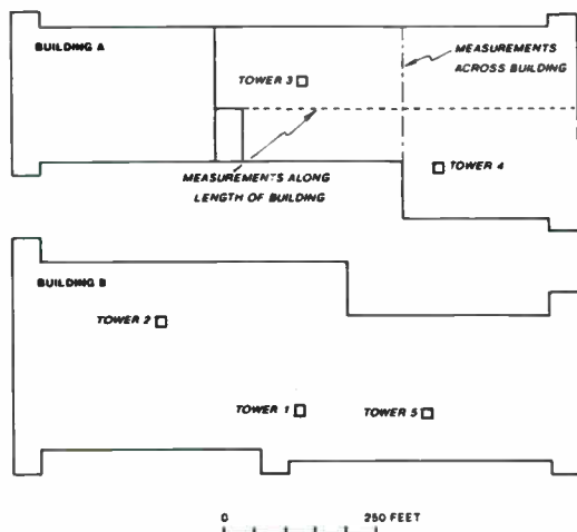
Figure 3. MEASUREMENT LOCATIONS TO DETERMINE EFFECTIVENESS OF SHIELDING
