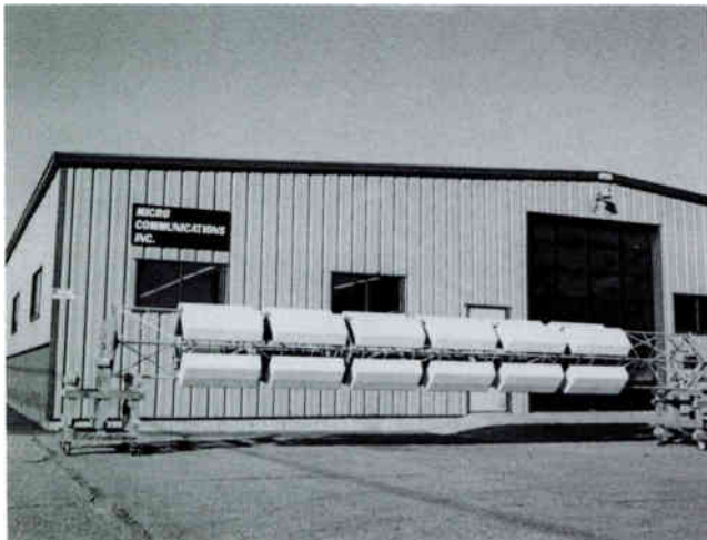
Fig.7 Six Bay Array Antenna
