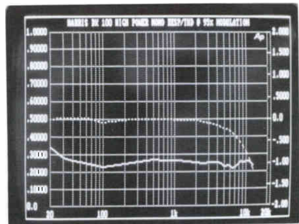
Figure 9 DX300 Distortion & Frequency Response 300 Kw Output (Lower curve distortion)
