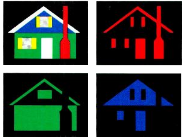
Fig. 10. Illustrating how a typical color image (upper left corner) can be separated by optical means into red, green, and blue counterparts.
