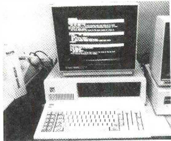
Fig. 3. A desk-top computer system with internal floppy disk and hard disk storage exceeding ten million BYTES. With newswire service input, this system can give a single user most of the functions of a multi-terminal newsroom computer system. Connected to a data communications network, it can perform as a full-featured newsroom workstation. (Courtesy of Basys, Inc.)
