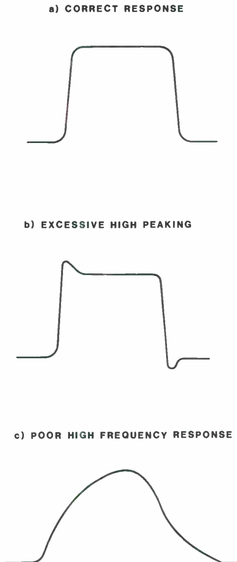
Fig. 33. Effect of frequency response on the reproduction of a white bar.
