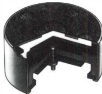
Fig. 5. Cutaway drawing of an electret condenser microphone element.
