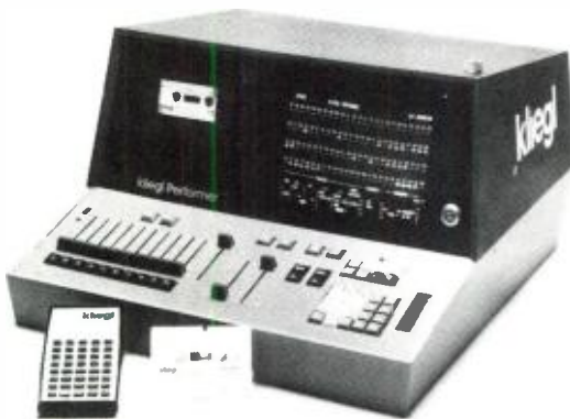
Fig. 21. Midsize light computer with single display can program complex cues and can drive a convenient hand-held remote unit. Data cassettes provide library storage of all settings. (Courtesy of Kliegl Bros.)
