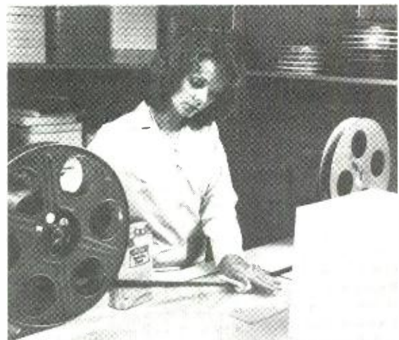
Fig. 10. Cleaning a film using a plush pad and a pair of rewinds.
