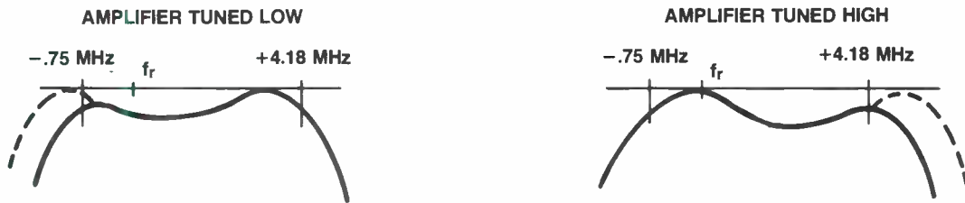
Fig. 65. Nonsymmetrical response caused by the amplifiers outside the transmitters bandpass. Solid line is transmitter overall response. Dotted line is the part of PA response outside of the transmitters bandpass.
