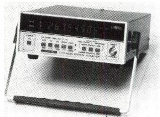
Fig. 1. A general purpose frequency counter may be used to measure carrier frequency as well as other frequencies within its range. Specified accuracy and resolution for the model shown here make it suitable for measuring carrier frequencies of AM, FM and VHF TV. (Courtesy of Leader Instruments Corp.)
