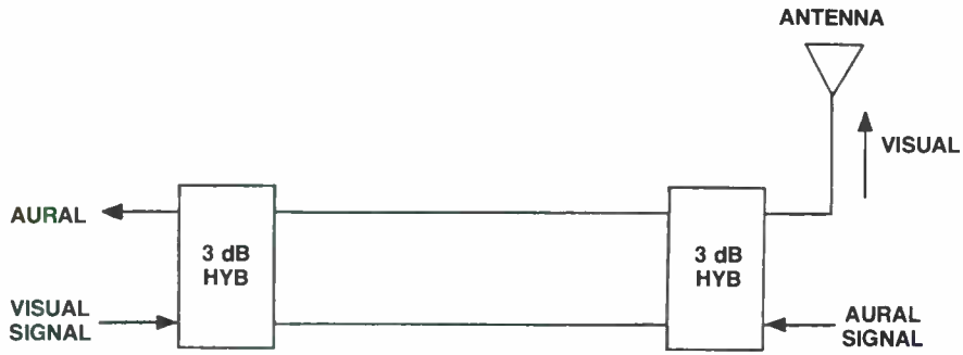
Fig. 77. Aural signal applied to back-to-back hybrids.
