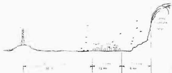
Fig. 2. Example of poor station location causing severe multipath propagation.
