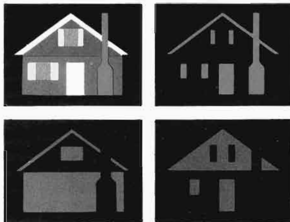
Fig. 10. Illustrating how a typical color image (upper left corner) can be separated by optical means into red, green, and blue counterparts.
