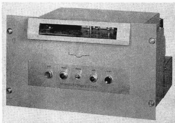
FIG. 4-2. Cartridge type of tape transport. (Courtesy of Collins Radio Company.)
