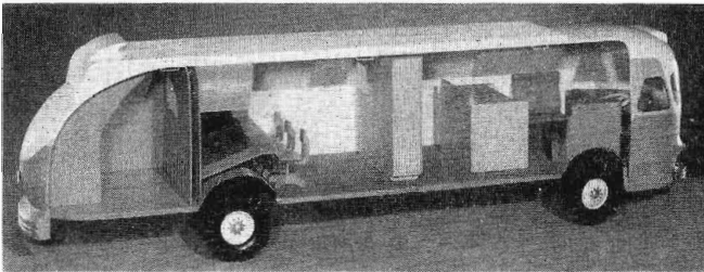
FIG. 5-16. Mobile TV tape system. The model shown here illustrates the manner in which one bus was outfitted as a mobile TV system, complete with tape recorder.
