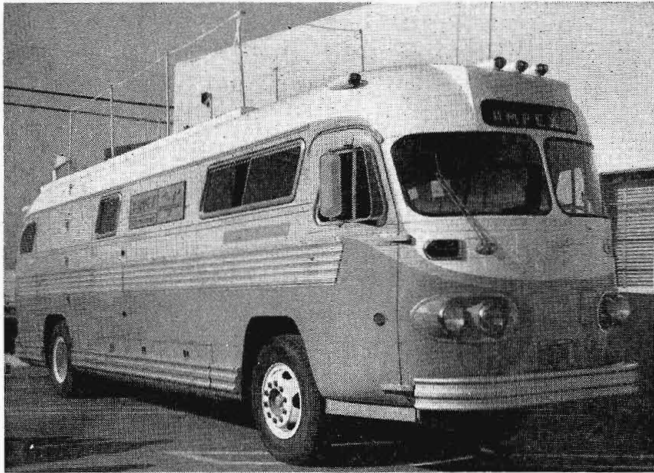
FIG. 5-17. A TV tape cruiser. Containing one video recorder, three cameras, centralized control facilities, and more than 10 kw of power-generating equipment, this air-conditioned cruiser covered more than 12,000 miles during the summer and fall of 1959, making recorded TV tapes "on the go" and on location.
