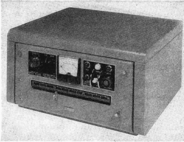
FIG. 4-3. Multiple-track tape transport. (Courtesy of Gates Radio Company.)
