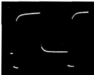
FIG. 5-59. Window signal—lows raised, highs raised—horizontal.
