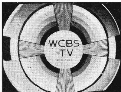
FIG. 5-91. Low resolution—receiver scanning spot too large.
