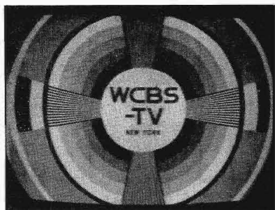
FIG. 5-89. Low resolution—roll-off from 1 Mc.
