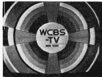
FIG. 5-68. Negative streaking-test pattern.
