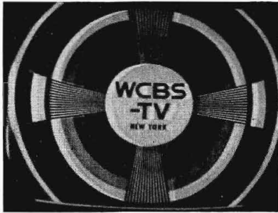
FIG. 5-102. Negative echo-test pattern.
