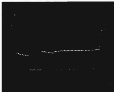
FIG. 5-75. Smearing—test pattern—expanded vertical.
