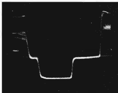
FIG. 5-90. Low resolution—roll-off from 1 Mc—expanded horizontal.
