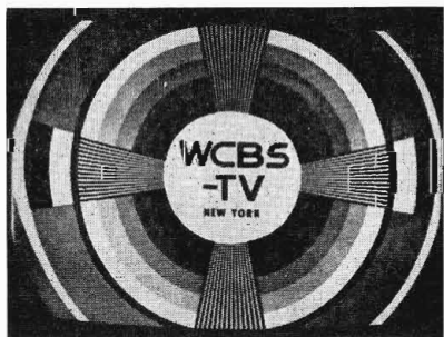
FIG. 5-76. Low setup—test pattern.
