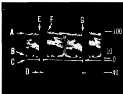
Fig. 5-2. Unimpaired video signal—A-scope horizontal presentation. A . White peak. B . Black peak. C . Blanking level. D . Synchronizing level. E-G . Complete horizontal interval = 63.5 \mu sec. E-F . Horizontal blanking interval = 10.05 \mu sec. F-G . Picture signal = 53.45 \mu sec.
