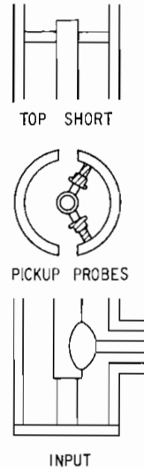
FIG. 7-41. Cross section of traveling-wave antenna at input, aperture, and top.
