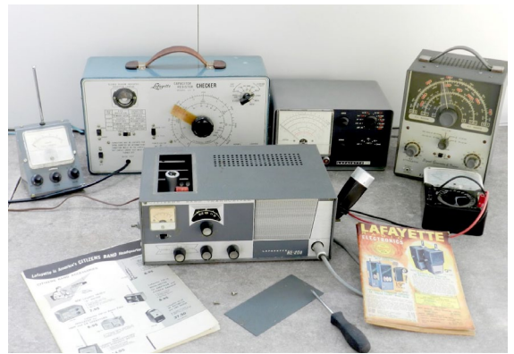
An all-Lafayette test-bench: Equipment from left: TM-16A field strength meter; LC-4 Capacitor-resistor checker; Model 174 VTVM; KT-208 signal generator and tracer; 30,000 ohm/volt VOM model 99-5004.
