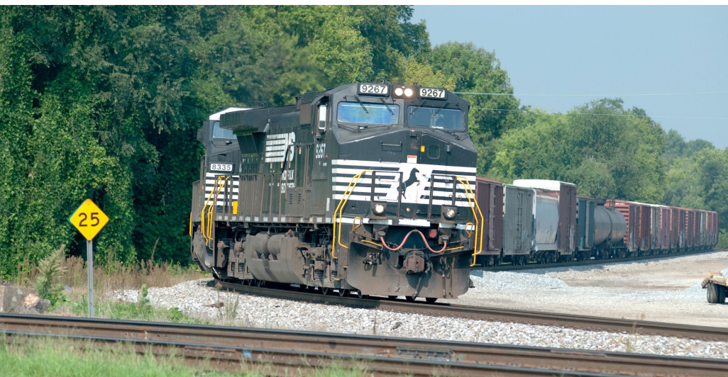
An eastbound Norfolk Southern (NS) merchandise train approaches the merger of the NS and CSX lines in Decatur, Alabama. Though the 25 mph speed board visible at the far left of the photo applies to the CSX line, both lines have sharp curves in the area, which limit train speeds.
