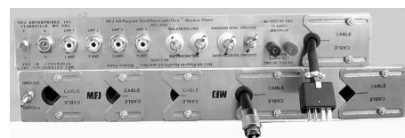
MFJ-4605 two-tiered feed-through ($160) offers connectors in addition to whole cable feeds. Construction is the same as the other MFJ products. (Courtesy: MFJ Enterprises)
