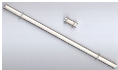
UG-363 Bulkhead 5/8 inch feed through will accept a PL-259 connector at both ends and comes in lengths from 1 inch ($2) to 12 inches ($19). Use individually or several in a piece of wood for a DIY multi-antenna window feed-through. (Courtesy: Universal Radio)
