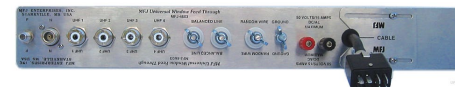
MFJ-4603 antenna feed-through ($80) is the deluxe version of the other two models. With the same wood, this model includes SO-239 jacks for HF/VHF, an N connector for VHF/UHF, one F connector for satellite TV, a balanced line twin feed on ceramic insulators, a random wire feed on a ceramic insulator, a ground wire connectors, a set of DC binding posts and a rubber-grommet channel for a rotator control cable (Cinch-Jones plug shown is not supplied). (Courtesy: Universal Radio)
