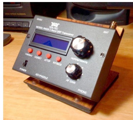
Ten-Tec R4020 – a two band CW transceiver made in China to Ten-Tec specs and backed by Ten-Tec. The 4020 covers 40 and 20 meters plus 5-16 MHz shortwave for $250 and is ready for action out of the box. (Photo courtesy of the author)
