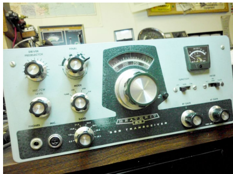
A front view of my Heathkit HW-100, minus the enclosure. It features a nice aftermarket dial modification
