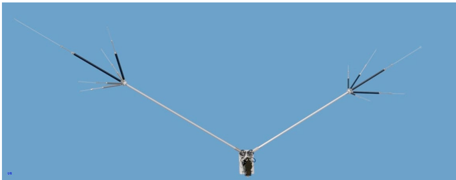
Comet CHV-5X ($320) rotatable dipole is only 13 feet across and covers 40 through 6 meters. Use it for restricted locations where using a full-sized dipole is not possible. (Courtesy: Universal Radio)
