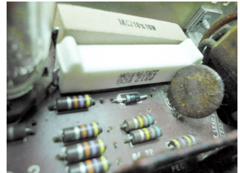
The scene of the crime on the audio circuit board, shown after the replacement of both stone resistors and the diode. When plugged in, these two resistors get very hot, thanks to a short farther down the line.
