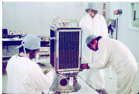
Technicians clad in their clean room "bunny suits" prepare UoSAT-2 for shipment to the launch site. (Courtesy: AMSAT-UK/SSTL)
