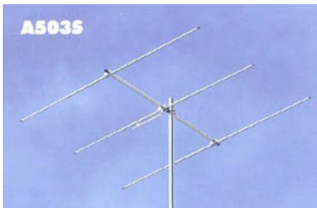
CushCraft A50 3S ($130) 3 element beam for 6 meters is light weight (just 7 pounds), has a boom length of just 6 feet and has 8 dB gain over a simple dipole. (Courtesy: Universal Radio)
