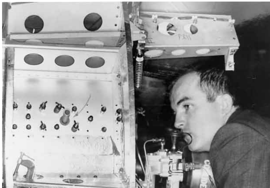
Lance Ginner, K6GSJ, looks over the carrying structure that will loft OSCAR-1 to orbit on the CORONA upper stage. Note the faint arrow pointing to OSCAR-1’s $1.15 Sears-Roebuck spring ejection mechanism. (Courtesy: K6GSJ)
