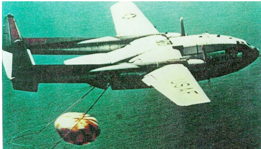
Exposed CORONA film was wound into its upper stage capsule that was later de-orbited and most often snagged in mid-air over the Pacific Ocean by a USAF C-119 cargo plane. (Courtesy: USAF)
