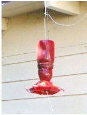
Closeup of IW5EDI's ingenious hummingbird feeder antenna for 40-10 meters.
