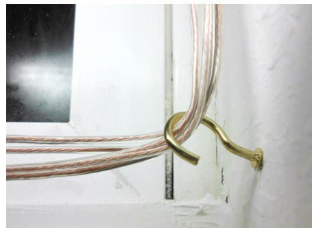
Four hook screws (adhesive coax clips would also work) like the one shown is all you need to run wire for a window loop antenna.
