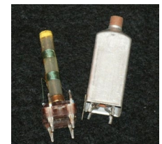
Coupled coils in an IF transformer
