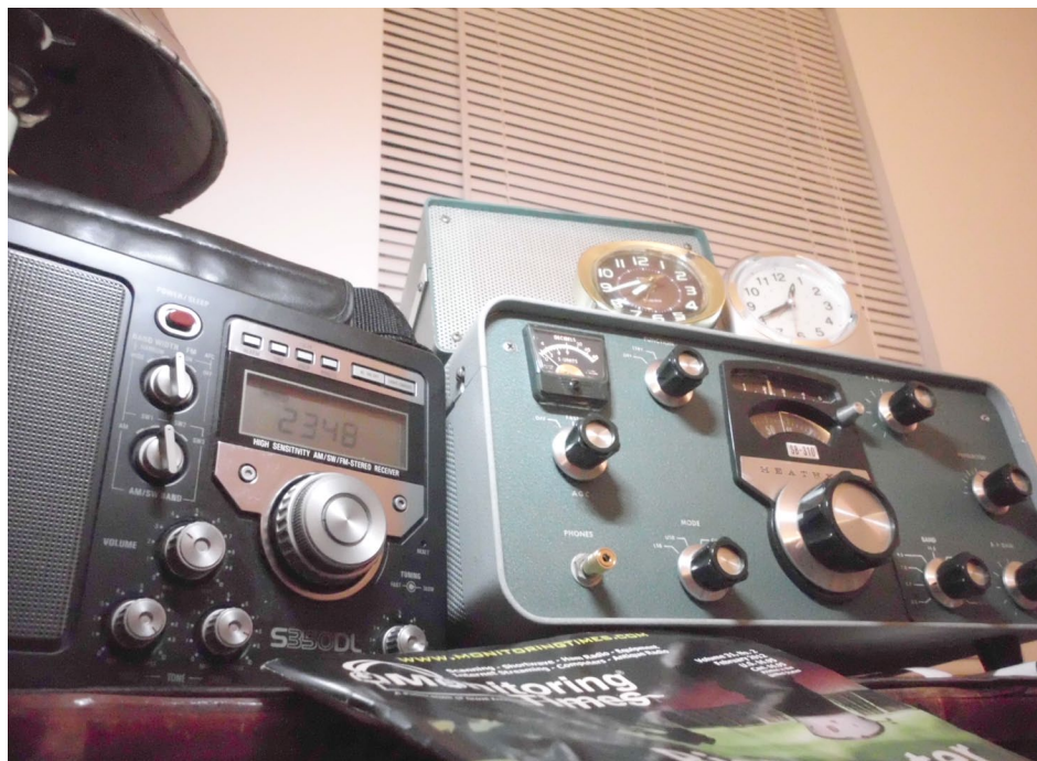
So, where's the antenna in this picture? There is more than 65 feet of wire antenna hidden behind the blinds!
