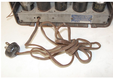
Check your line cord carefully. Chances are it's quite brittle and crumbly even if it seems intact.
