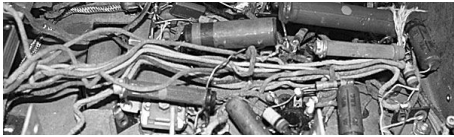
The remains of a cable in the parts set after it was taken apart to trace the BFO B+ lead. I'm glad I didn't have to do this to the restored set!
