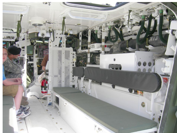
Inside view of troop carrying cabin. Most of the comms equipment is lined up along the right side, at about head height.
