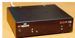
The RFSpace SDR-IQ, a software-defined radio that works with Sigmira.
