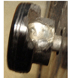
Fig. 2. It required extensive drilling and the ruin of about five drill bits to separate the bandswitch knob from the shaft.
