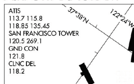
This is the corner of the airport diagram for San Francisco International (KSFO) which shows the airport frequencies.
