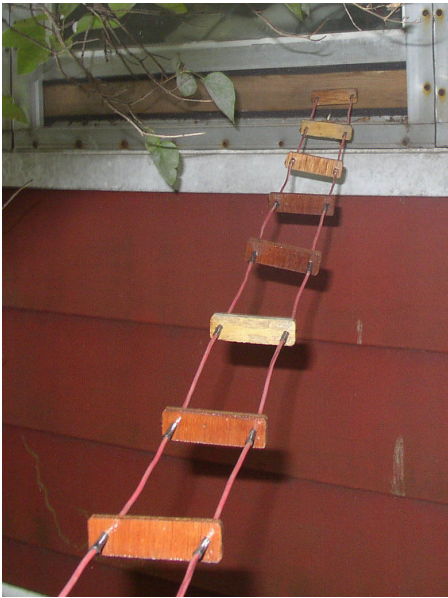
From the shack window, the feedline passes an antenna tuner "doghouse" ...
